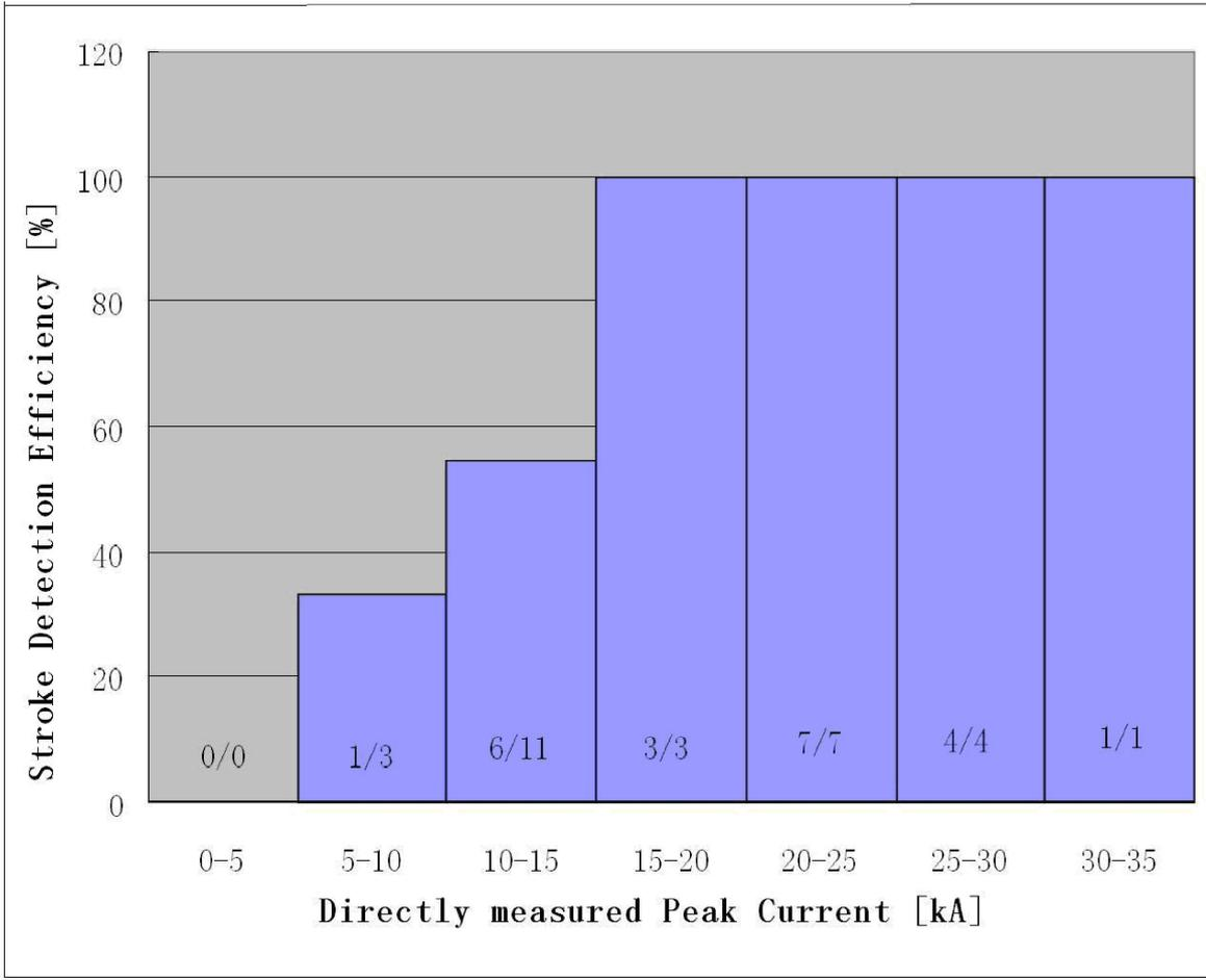
The arithmetic mean values of the flash detection efficiency and stroke detection efficiency were around 94%, 60% respectively.
