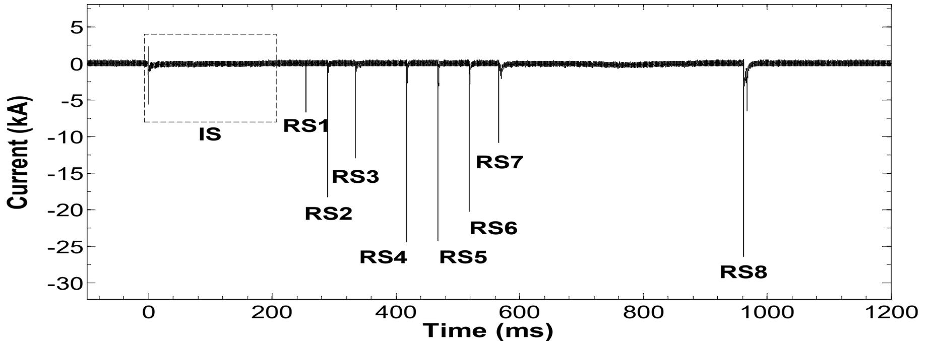
Channel-base current waveform of T200804
