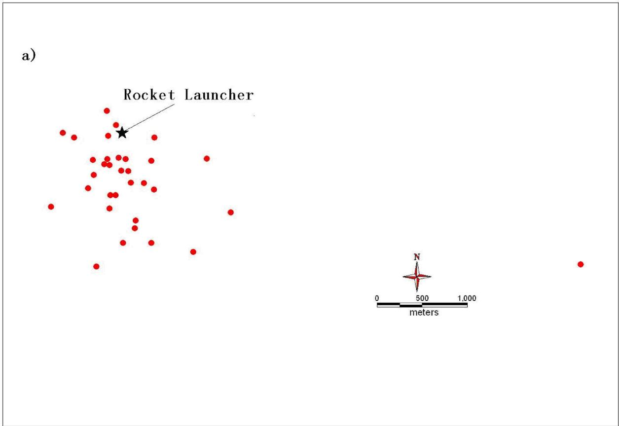
33 strokes in classical-triggered lightning were detected with more than 2 reporting sensors Locating accuracy ranged from 111 to 5,250m, with mean value of 710m
