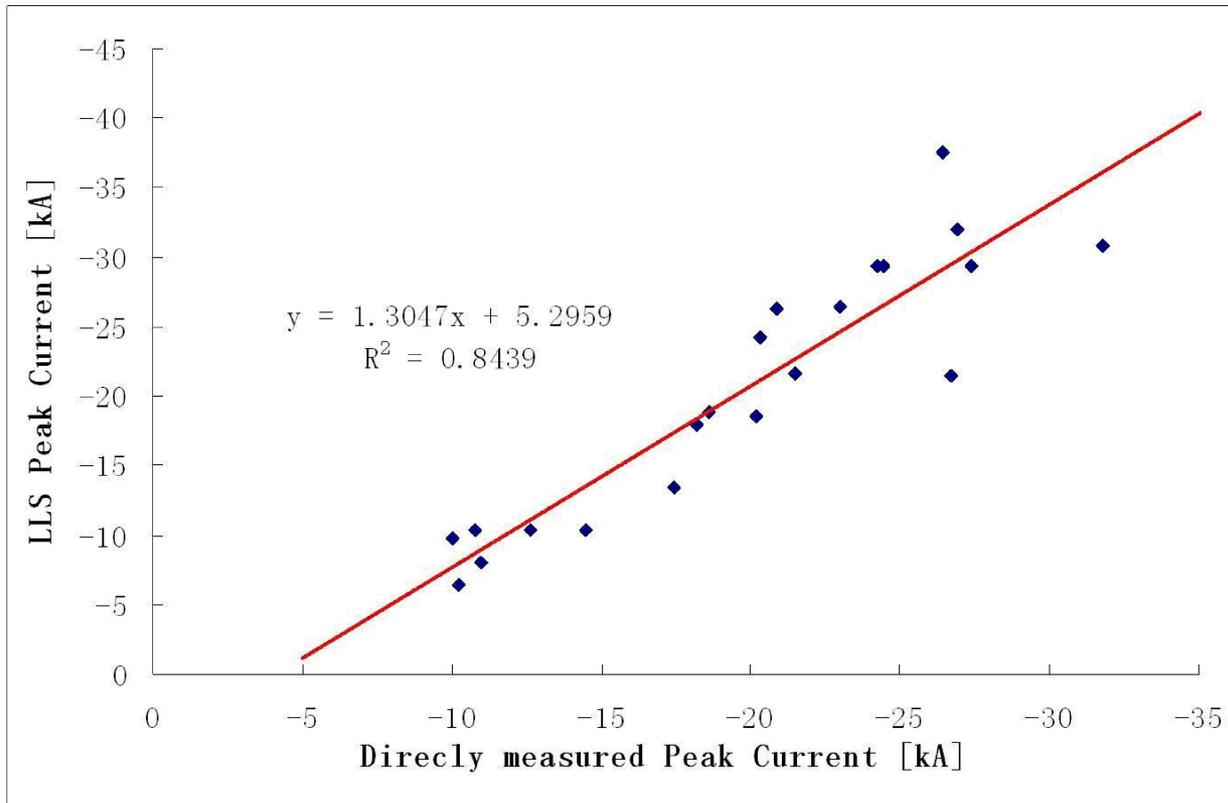
From 2008 to 2011, for 22 return stroke processes of artificially triggered lightning, both the directly measurement of peak currents and the corresponding LLS records were obtained.
