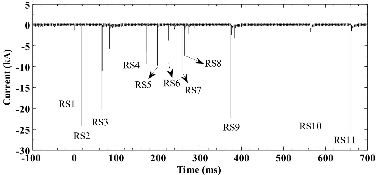
Channel-base current waveform of T201404 (except the return strokes; the others were M-components)
