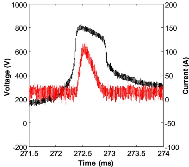
Residual voltage waveform (black lines) of the SPD1 and the corresponding current waveform (red lines) flowing through the SPD1 during two minor M-components (3,5kA) in T201404.
