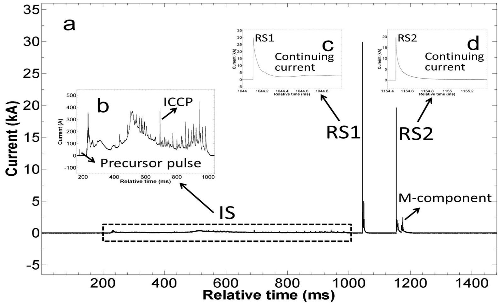
An example of the current waveform of a classical TLF (T150612161626). (a): Whole current waveform. (b): The IS current. (c) and (d): **Partial enlarged details** of the first and second RS current waveforms **and the following continuing currents**, respectively. The current waveforms shown in a, c, and d were recorded using the channel with a  $\pm 50$  kA measuring range, whereas that shown in b was recorded using the channel with a  $\pm 2$  kA range. ICCP: Initial continuous current pulse.
