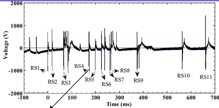
The voltage waveforms between two terminals of the SPD1 during T201404.
